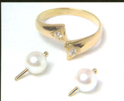
Some delicate designs would be impossible without a laser welder. Manufacturers who don't own lasers can contact service bureaus to complete their visions. Here, Bob Staley used a laser to assemble this ring for a client. Using a torch to solder the components would have damaged the pearls.
