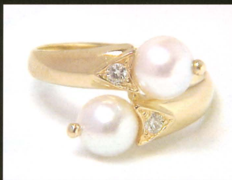
Some delicate designs would be impossible without a laser welder. Manufacturers who don't own lasers can contact service bureaus to complete their visions. Here, Bob Staley used a laser to assemble this ring for a client. Using a torch to solder the components would have damaged the pearls.
