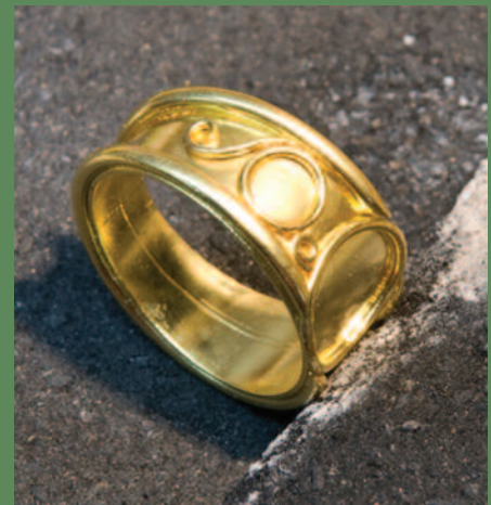
⤴ 4. The base shape for the piece, a 22k ring shank, is fabricated and wires are fused to its edges and within open areas. The wire will act as a base to support the granules, enabling them to be fused not only to the base metal but also to the wire, anchoring them more securely to the piece.
