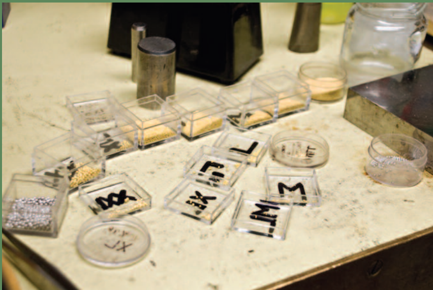
⤴ 3. The Gualtieris make thousands of granules twice a year, estimating how much they will need in each metal used to build stock and fulfill custom orders. They sort the granules through mesh scientific sifting screens to calibrate them, and store them by size and alloy.
