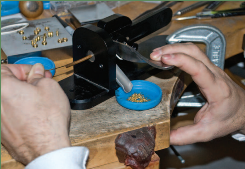
THE PROCESS ⤴ 1. To make granules, the Gualtieris begin by cutting tiny bits of wire—22k yellow gold is shown here—into uniform sizes. This process is made easier by the use of a special granule cutter that resembles a paper cutter.
